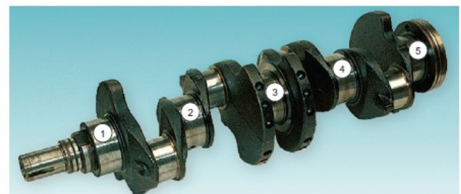
Figure 2.75 Crankshaft: 1-5 main journals
