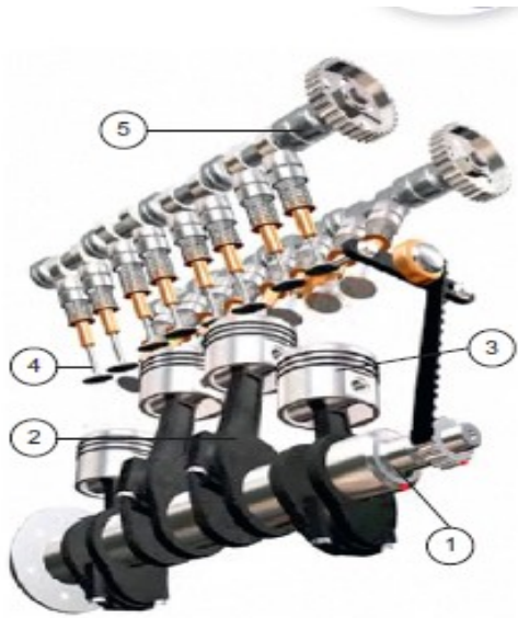
Figure 2.1 Internal combustion engine internal components: 1, crankshaft; 2, connecting rods; 3, pistons; 4, valves; 5, camshafts
