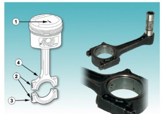
Figure 2.69 Con rod features: 1, front of engine; 2, identification marks; 3, big end cap; 4, oil spray hole for cylinder wall lubrication
