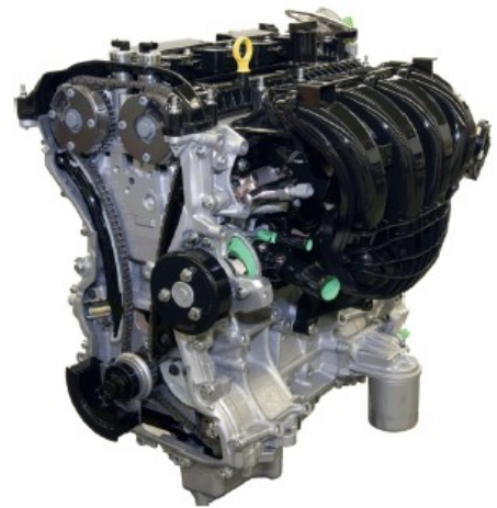
Figure 2.51 Engines vary, here is a four cylinder inline design. (Source: Ford Media)
